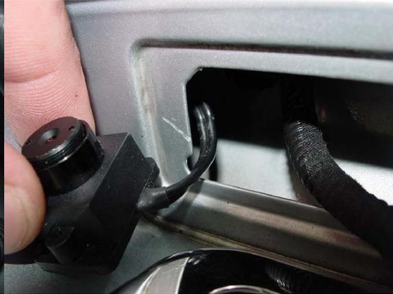
run wires from the right (battery) compartment to the left (Video Module)
